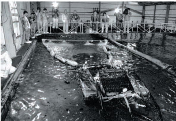
Fig 4. 18 Tank test of the oil skimmer installed the oil raking system
