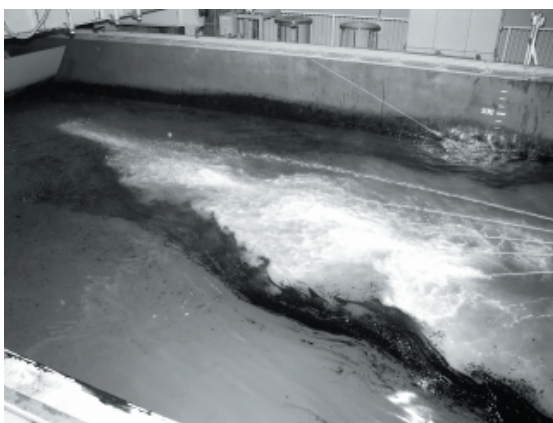
Fig 5.30 Oil gathering by water jet stream
