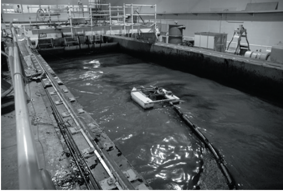
Fig 5.44 Tank test of the buoy model (II) changed towing point in STORMS
