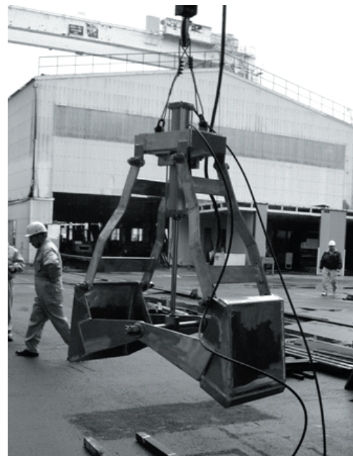
Fig 5.7 1/4 scale model of the grab bucket
