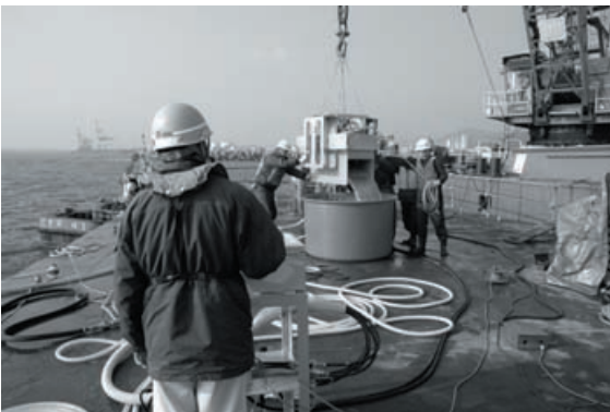
Fig 5. 65 Scoop the seawater and discharge into the storage tank. Operator is nearest man.
