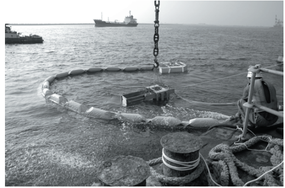
Fig 5. 64 Operation of the Bucket oil skimmer with rake model
