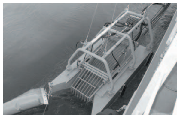
Fig 4.25 The net conveyor skimmer installed by the side of Dr.Kaiyo
