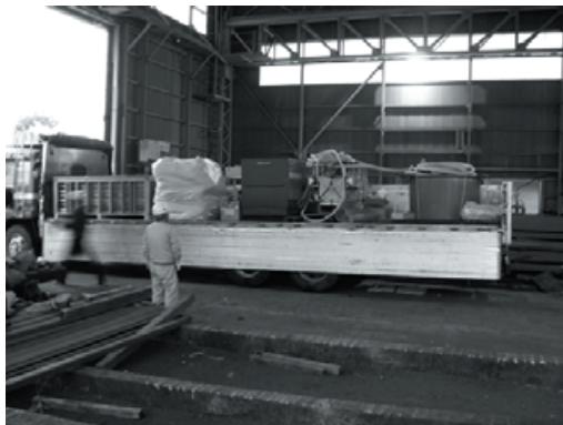
Fig 5. 49 The oil recovery system package on the 11 ton class truck bed
