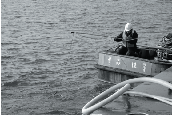
Fig 5. 63 Measure the current velocity (near the thruster)
