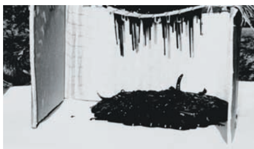
Fig 4.3 Time test of high viscous oil passing through nets
