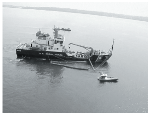
Fig 5. 22 Collecting boom (outrigger type ; USCG)
