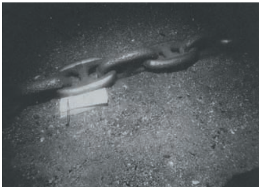
Fig.2.11 Measurement of mooring facility of lighted buoy (Tokyo Bay).
