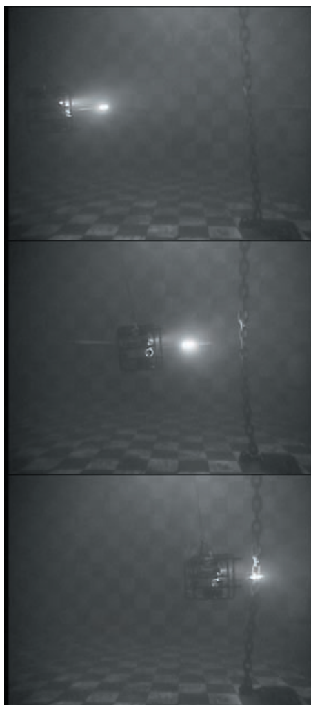
Fig.4.28 Appearance of the target capturing and vehicle navigation under the wave condition.
