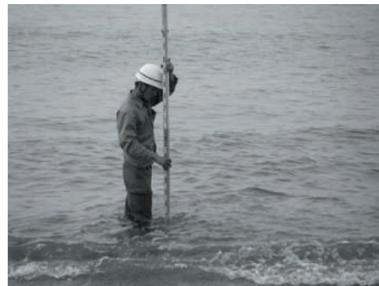
Fig.2.10 A worker with staff who walk into surf zone (Niigata West Coast).
