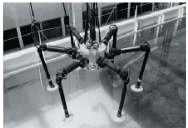
b) Aqua-robot 3 (Light & watertight type test model; 280kg)
