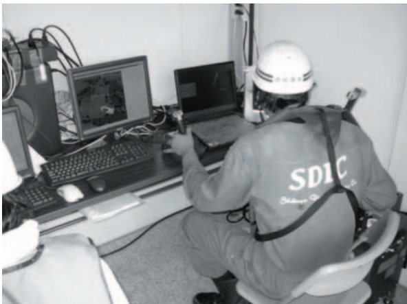
Fig.2.4 Teleoperation type underwater backhoe using haptic image.
