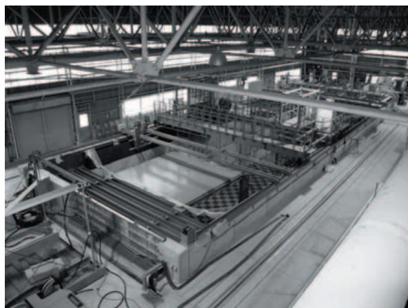
Fig.4.20 Simulation tank for underwater working environment.
