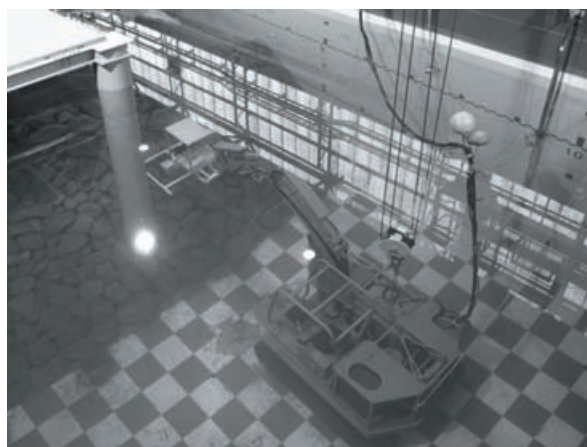
b) Test of contactless thickness measurement system equipped on a teleoperated underwater backhoe (water level; 6m)
