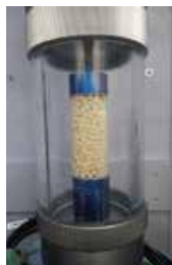
Compression test on a simulated specimen having the identical particle structure
