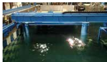
ROV for inspecting pier superstructures and its experiment in a water tank (with wave and current)
