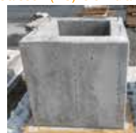
Experiment on concrete made of high-density recycled aggregate (copper slag fine aggregate) (The concrete was produced at an actual plant and then transported and placed using a concrete pump)
