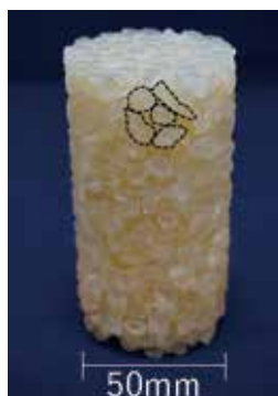
Simulated test specimen that has been 3D-printed using gravel material
