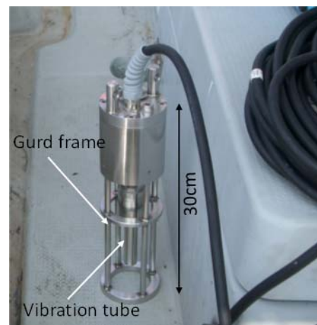
Figure 2.7 Sensor of in-situ mud density measurement
