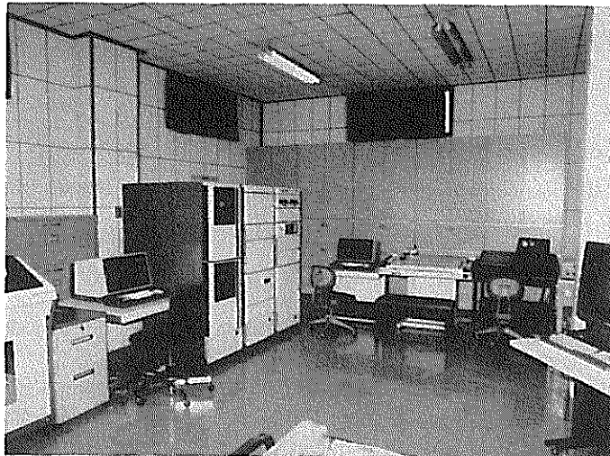
Fig. 25 Hybrid computer controlling the digitizer
