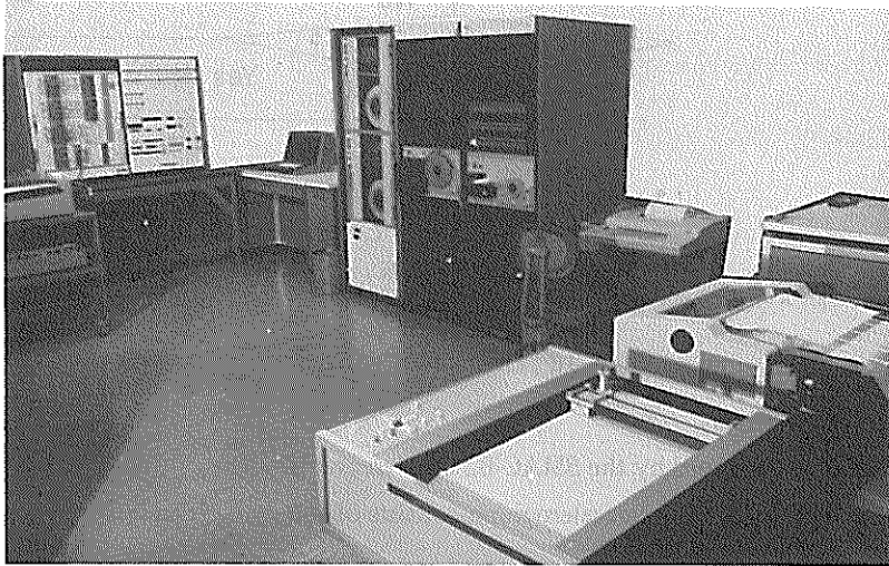
Fig. 15 Hybrid computer controlling the digitizer
