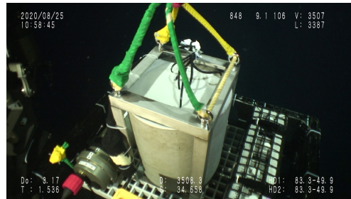
Fig. 12 Mortar specimen and apparatus for in-situ measurement during the dive to the deep sea experimental field location at Nankai Trough.
