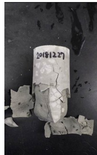
Fig. 1 Illustration of the rupture of the cement-based specimen due to water transport and confinement under high hydraulic pressure ( left ). Hardened Portland cement paste that was pressurized from 0.1 MPa to 60 MPa at a pressurizing rate of 1 MPa/min, and the 60 MPa was maintained for 60 min, then depressurized from 60 MPa to 0.1 MPa at a depressurizing rate of 1 MPa/min ( right ). The original shape of the hardened paste was 50 mm in diameter and 100 mm in height.
