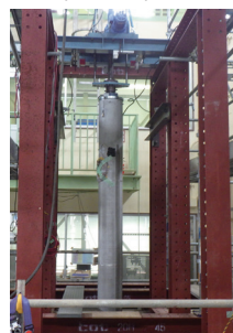
Horizontal loading experiment involving a large-diameter pile
