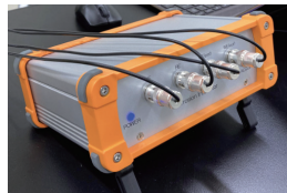
Figure 1: Corrosion diagnosis unit incorporating the new method
