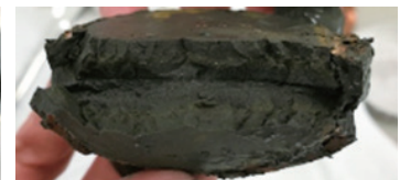
Clay sample from Tokyo Bay, before and after the electro-osmotic consolidation and dehydration test
