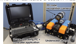
Underwater drone used in the experiment
