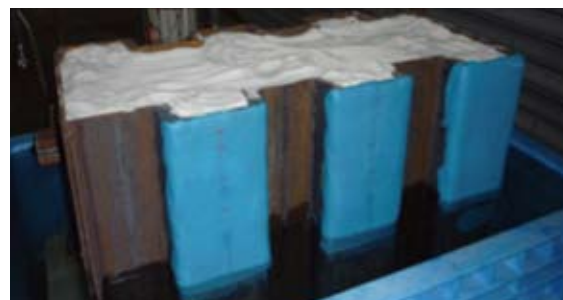
Steel sheet pile specimen
