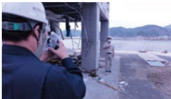
State of investigation of the run-up height by a range finder
