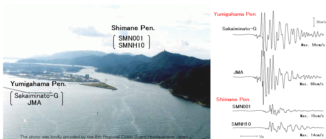
Figure 2 The topography around the port of Sakai, west Japan (left) and the velocity waveforms for the fault-normal component recorded around the port during the 2000 Tottori-ken Seibu earthquake ( M_j7.3 ).
