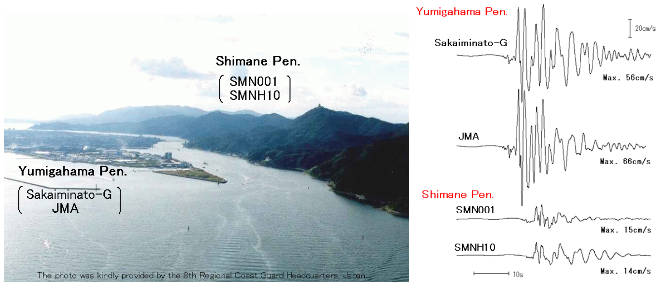
Figure 2 The topography around the Port of Sakai, western Japan (left) and the velocity waveforms for the fault-normal component recorded around the port during the 2000 Tottori-ken Seibu earthquake ( M_J7.3 ). The peak ground velocities observed in the plains of Yumigahama Peninsula were approximately four times larger than those observed in mountainous Shimane Peninsula.
